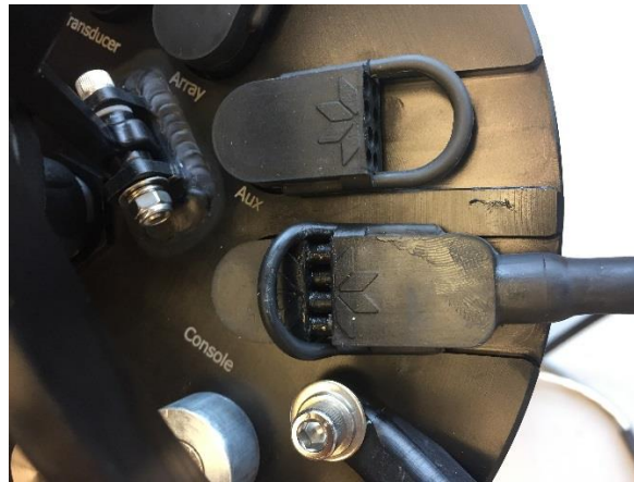
Figure 12 Console cable with locking strap removed (partially installed)
