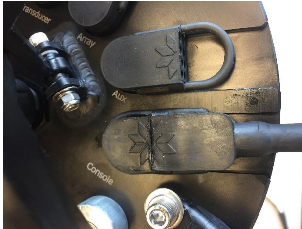
Figure 13 Fully installed console connector with locking strap installed
