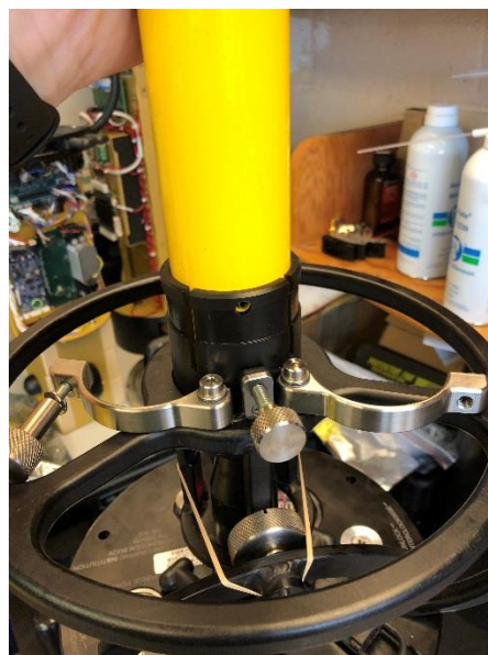
Figure 6 Antenna Aligned with rotational locking screw
