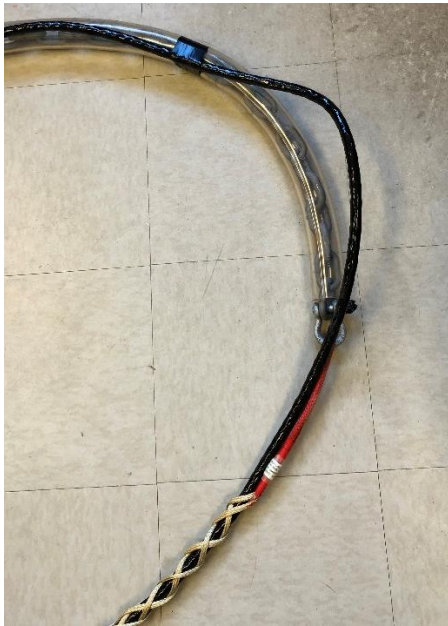
Figure 23 proper mating of YaleGrip to transducer cable and buoy chain
