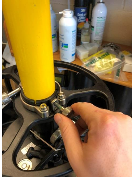
Figure 7 Insert rotational locking screw
