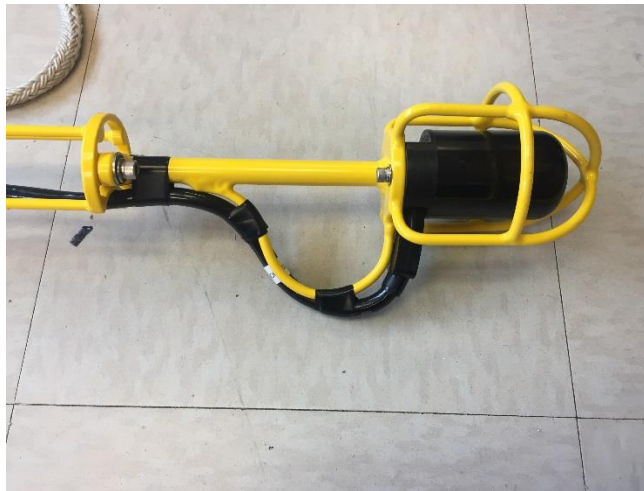
Figure 26 Properly mated 25KHz transducer and transducer cable
