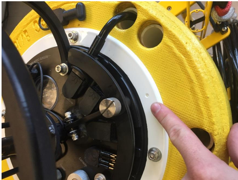
Figure 19 endcap is properly seated and twist lock is aligned and locked
