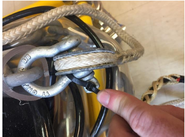
Figure 24 Properly secured screw pin shackle using cable tie
