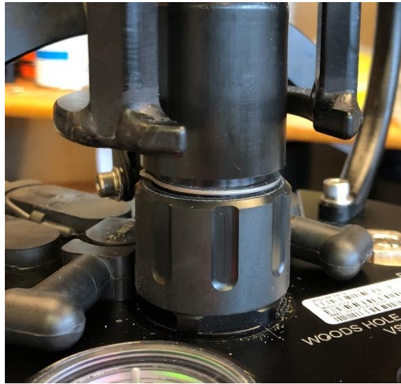
Figure 9 Fully installed Quad RF connector
