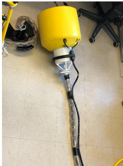
Figure 22 Proper mating of cable to surface buoy
