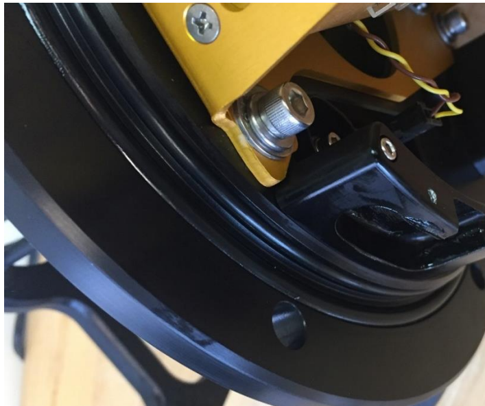
Figure 16 Proper O-ring seating and Lubrication
