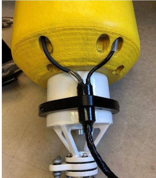
Figure 21 Proper installation of transducer cable to hull
