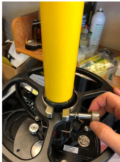
Figure 8 Close and tighten thumb screw to lock mast in place
