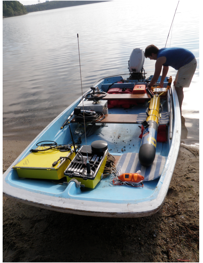
Fig. 6. Iver2 AUV and Wave Glider command and control module and acoustic communications payload module being readied for deployment in a local lake.
