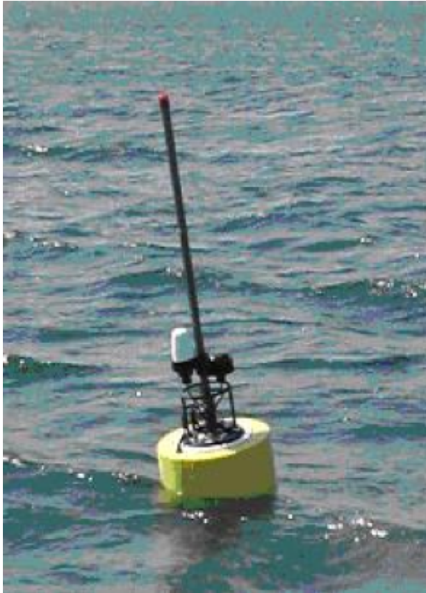
Fig. 4. Micro-modem based RF / Acoustic Gateway Buoy, with modem and Freewave serial radio
