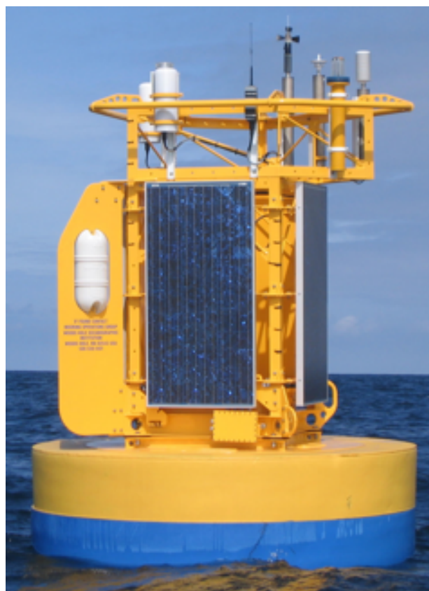
Fig. 11. The Nootka Observatory Buoy, with meteorological sensors and solar panels.
