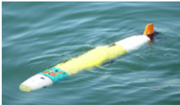
Fig. 7. The lightweight shallow water REMUS AUV (developed at WHOI), with Micro-modem for acoustic telemetry and remote control.
