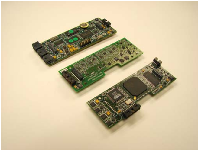
Fig. 3. Micro-Modem main board (top), Multi-channel analog board (middle) and floating-point co-processor card (bottom).
