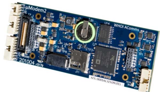
Figure 1. The 4.5" x 1.75" Micromodem-2 preserves the physical form factor of the Micromodem-1 while providing improved expansion connectors and I/O capabilities.
