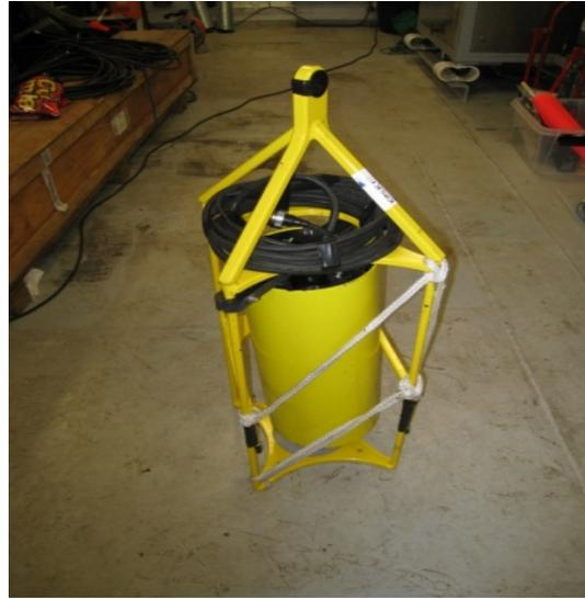
Figure 5 900 Hz Helmholtz resonator used for the Fram Strait experiment and deployed to 100 m at each station.
