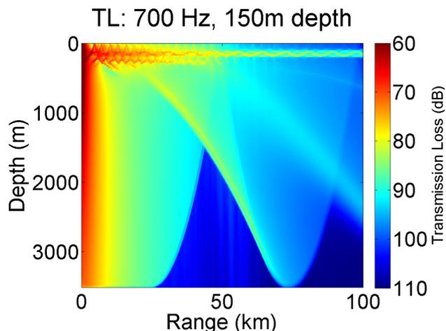
Figure 14 TL for a 150 m source showing the resulting ducted energy.
