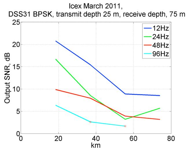
Figure 17 SNR at the output of the adaptive equalizer for the 25m-75m transmit-receiver depth case.
