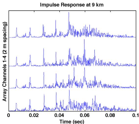
Figure 4. Measured impulse response at 7 kHz carrier with 4 kHz bandwidth FM sweep.
