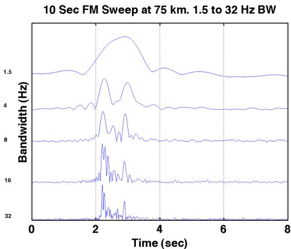
Figure 15 Matched-filter of sweeps of 1.5 to 32 Hz bandwidth (top to bottom) at the maximum range during the ICEX 2011 experiment.
