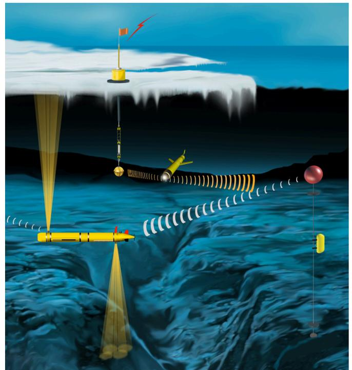
Figure 1. Gliders and powered AUVs performing oceanographic work beneath the Arctic ice.
