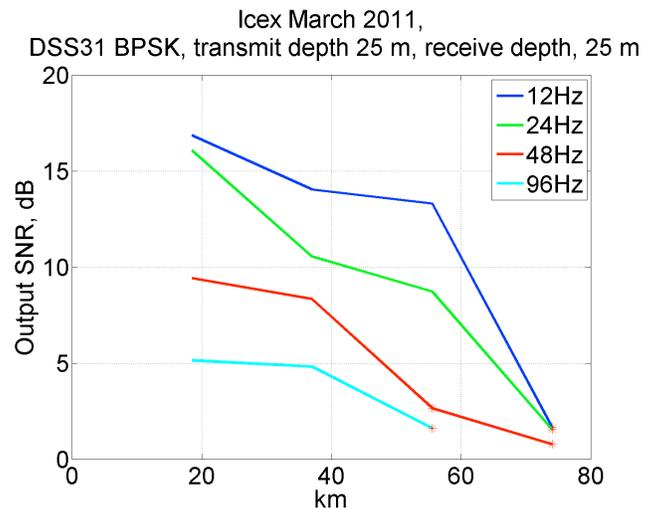
Figure 16 SNR at the output of the adaptive equalizer for the 25m-25m transmit-receiver depth case.
