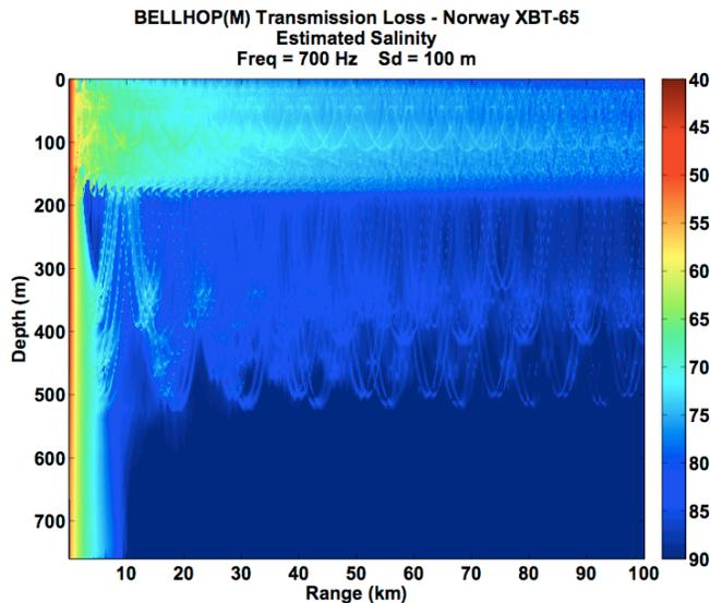
Figure 8 Transmission loss for the Fram Strait, Sept. 2010.
