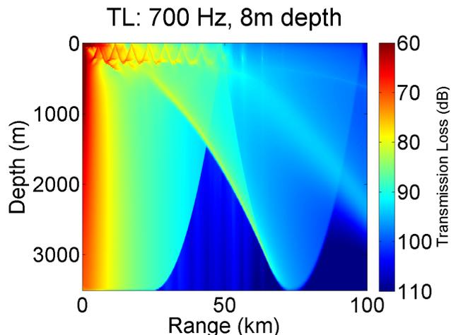
Figure 13 Transmission loss corresponding to the 2011 sound speed data. A loss-less surface reflection is assumed for simplicity.
