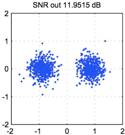
Figure 10 Single-channel equalizer result at 40 km
