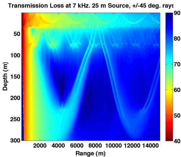
Figure 3. Transmission loss for a shallow source (25m).
