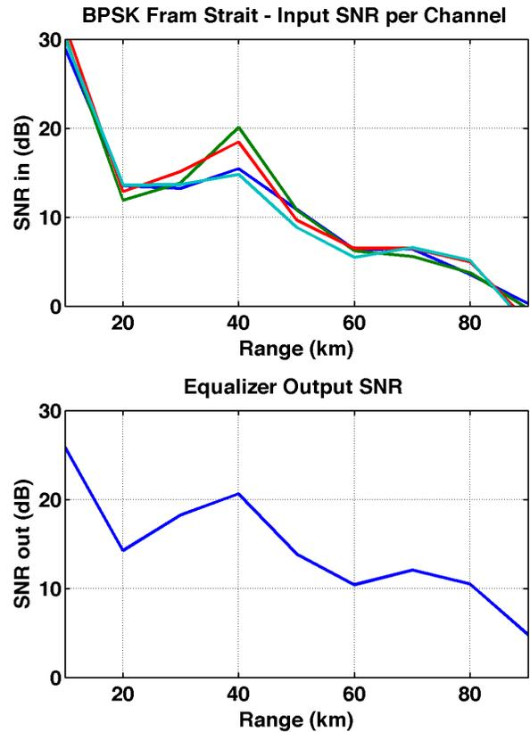
Figure 9 Fram Strait input and output SNR for a 12 Hz BPSK signal.
